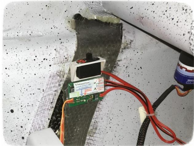
**Installation and connections must be done with the mechanical activation switch in 'OFF' position and the RC reception system must be powered off for maximum security.**
